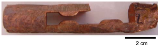
Fig. 11 Image of the ECAE consolidated 100 nm Cu powder following route 4B with all dimensions in the centimeter range. Several tension samples were cut from the middle of the billet
